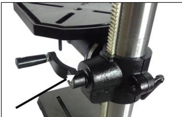
Figure 6-1: installing crank handle
